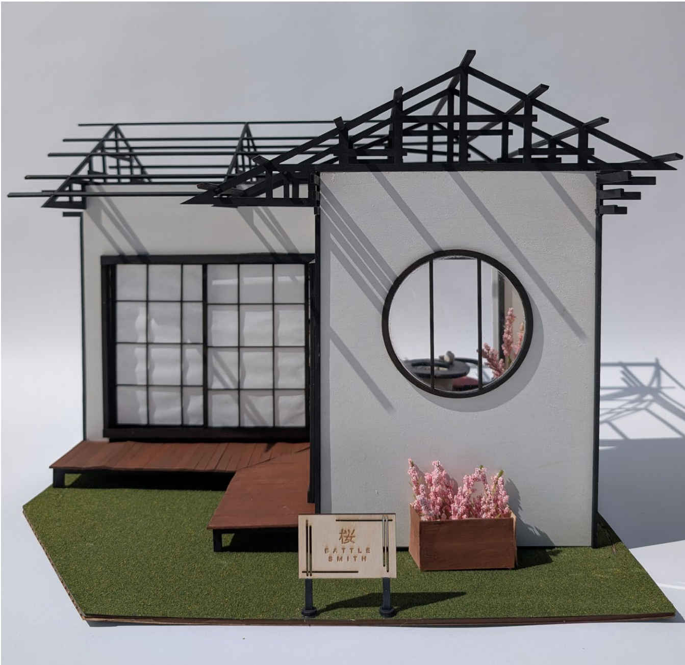
Model structure cut with laser on bass wood. Shoji paper installed in sliding doors and decking made from popsicle sticks. Constructed Model Exterior Perspective ————— Model Scale - 1:12
