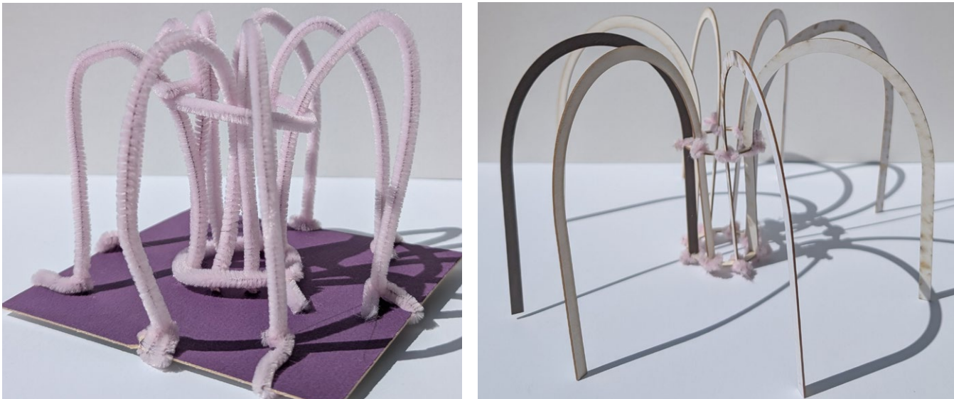
Early form studies using pipe cleaners and laser-cut matboard to test fastening methods and structural behavior through two iterative attempts. Schematic Study Models
